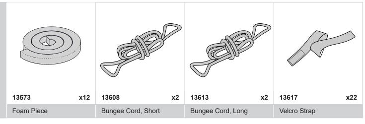
**EN** Insert the foam pieces into the pocket under the skirt of the mat and close the Velcro strips.
